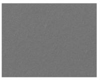
**TEEE:** Thermoplastic Elastomer Ethyl Ester – is a material that combines the flexibility of rubber with the strength of a membrane, resisting tears, abrasion and corrosion. It also has good resistance to surfactants.
