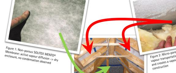
Figure 2: Micro-porous membrane: no active Vapour transportation -> condensation observed and creates a vapour closed film -> wet construction
