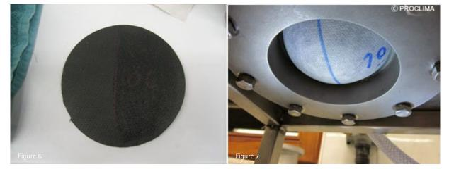
SOLITEX® range uses monolithic membrane and is waterproof (ISO 811) up to lab test limitation of 10 meters head of water. Right side is coated with oil without effect on waterproofness.
