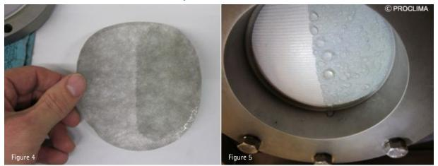
Lab test water column (ISO 811) on conventional WRB. The right half was treated with oil, rendering it leaky. The Australian and New Zealand building codes use a similar test method (AS 4201.4) which requires significantly lower test pressures (0.1m vs EN > 1m) and over different time cycles (24 hours vs EN 2 hours).
