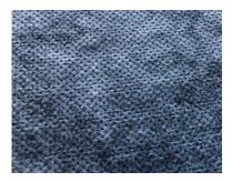
The **bottom microfiber fleece** protects the TEEE layer above from damage during construction.
