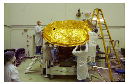
Figure 3: Low-emissivity surfaces are used in space where there is no atmosphere, and heat transfer is 100% radiative. (Image: NASA/JPL, 2019)
