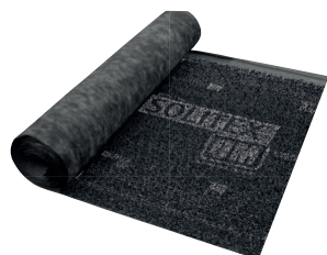
SOLITEX UM Four-layer underlay with 3D separation layer and self-adhesive strip
