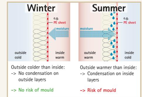
Fig. 30. The effects of a vapour barrier on the outside
