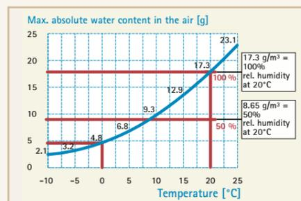
Air can hold different amounts of moisture, depending on its temperature.
