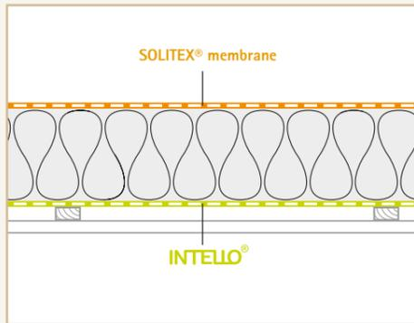
Advantages of covering the thermal insulation with wall wrap, pro clima SOLITEX membran:
