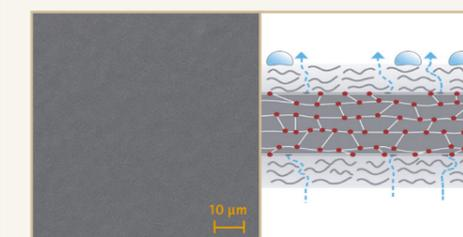
Microscopic detail of a non porous membrane Active diffusion transport
