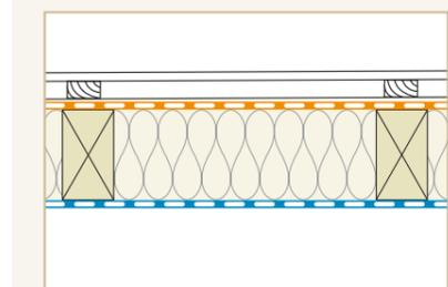
airtight on the inside and wind- and weathertight on the outside
