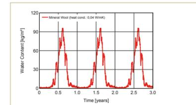
→ Moisture content of the 5 mm outer layer of thermal insulation rose to 90 kg/m<sup>3</sup>
