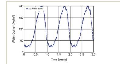
→ Moisture content of the cement-bonded boards rose to 240 kg/m<sup>3</sup>
