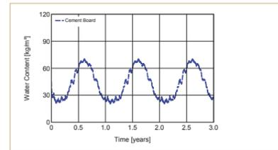
→ Moisture content of the cement-bonded boards rose to 70 kg/m<sup>3</sup>
