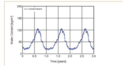
→ Moisture content of the cement-bonded boards rose to 120 kg/m<sup>3</sup>
