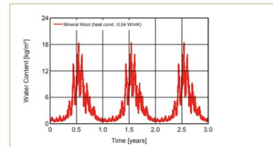
→ Moisture content of the 5 mm outer layer of thermal insulation rose to 18 kg/m<sup>3</sup>
