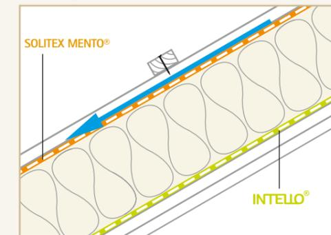
If there are rooms immediately under pitched roofs, the physical demands are similar to those for walls. The requirements for a well protected roof construction are therefore also similar to those for walls:
