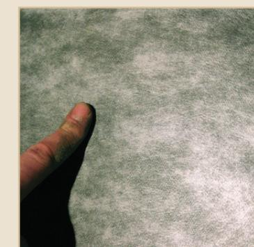
Nonporous SOLITEX TEEE membrane - Active diffusion transport: Dry - No condensation
