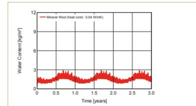
→ Insignificant increase in the moisture content of the 5 mm inner layer of thermal insulation
