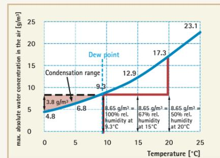
Under standard environmental conditions (20°C/50% relative humidity) the dew point is reached at 9.3°C. If the temperature drops to 0°C, 3.8 g/m<sup>3</sup> of condensation is deposited.
