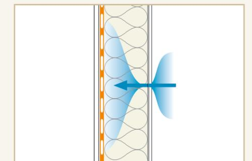
A significant amount of moisture can penetrate the building envelope by convection. This poses the risk of structural damage and mould if there is insufficient moisture compensation. The ideal solution is intelligent moisture management.
