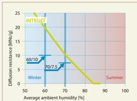
Adhering to the 60/10 rule and Hydrosafe™-value ensures a high potential freedom from structural damage for thermal insulation in new buildings and during construction.
