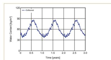
→ Moisture content of the 5 mm inner layer of wooden cladding rose to 80 kg/m<sup>3</sup>
