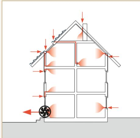
A fan creates low pressure in the building. Where there are penetrates, air enters the building from outside. These defects can then be put right relatively effortlessly.
