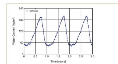
→ Moisture content of the 5 mm inner layer of wooden cladding rose to 190 kg/m<sup>2</sup>
