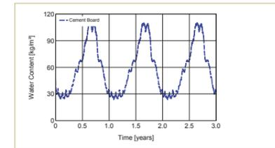
→ Moisture content of the cement-bonded boards rose to 110 kg/m<sup>3</sup>
