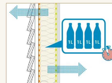
Four litres of water are added into the construction. The faster it can dry out (inwards and outwards), the higher its potential freedom from structural damage.
