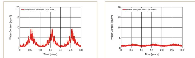
**Setup B: Diffusion resistance of the wall wrap: 2.50 MNs/g**
