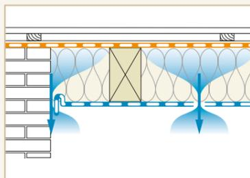
Non-airtight connection, the airtight building envelope is not continuous and closed
