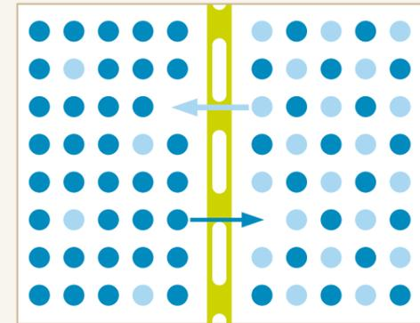
Moisture transport due to diffusion flow can be planned and allowed for.
