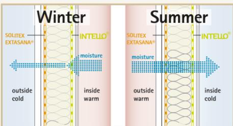
Due to the change in the diffusion resistance, intelligent airtightness systems can reduce the risk of structural damage and mould extremely effectively, both in the summer and in the winter.
