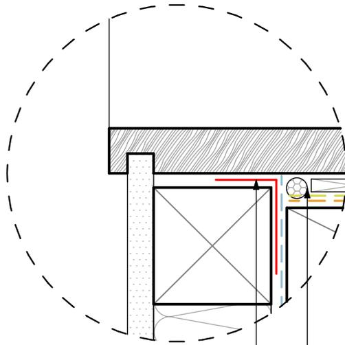
Stick Pro Clima TESCON PROFIL® to the back of reveal and over the Pro Clima INTELLO PLUS® vapour check to create an uninterrupted airtight seal around the window frame.
