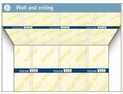
Lay the INTELLO® PLUS so that it completely covers the walls and ceiling and tape it with TESCON VANA, ensuring that you form an airtight seal.
