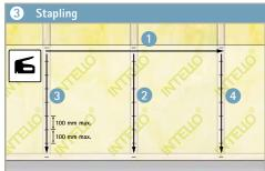
Staple along the entire upper edge of the INTELLO® PLUS (1) to every stud first, then on a middle stud (2). Run a hand down toward the floor to tighten the INTELLO® PLUS and ensure there is a 30 mm return for fixing to floor. Apply the first staples from the bottom. Leave a max. distance of 100 – 150 mm between each staple.
