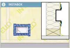
Cut a hole in the INTELLO® PLUS that is the same size as the INSTABDOX. Make the required number of holes in the INSTABDOX and feed the cable through these holes. Align the INSTAABOX and tape it to the INTELLO® PLUS with TESCON VANA, ensuring that you form an airtight seal.
