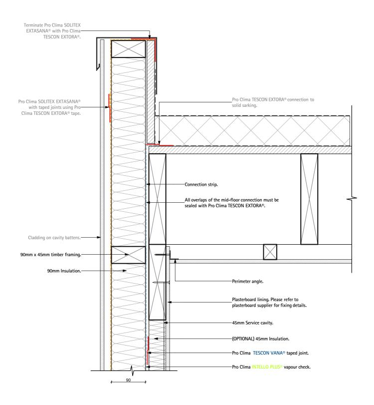
NOTE: Connection Strip must be installed during framing stage.
