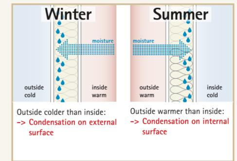
Fig. 29. The effects of a vapour barrier on the inside
