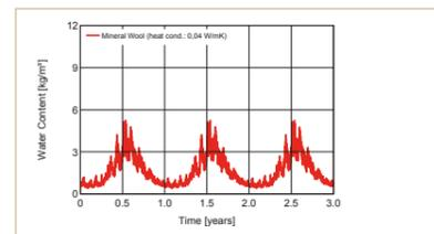
→ Moisture content of the 5 mm outer layer of thermal insulation rose to 5.5 kg/m<sup>3</sup>
