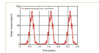
→ Moisture content of the 5 mm outer layer of thermal insulation rose to 100 kg/m<sup>3</sup>
