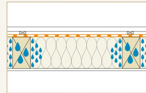
Building materials that are installed damp or that become wet or damp during construction have to be able to dry out without damaging the structure. The amount of moisture this involves is often underestimated.
