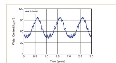
→ Moisture content of the 5 mm inner layer of wooden cladding rose to 100 kg/m<sup>2</sup>
