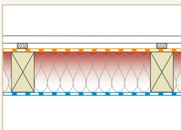
Airtight and windtight roof construction prevents heat flow by convection
