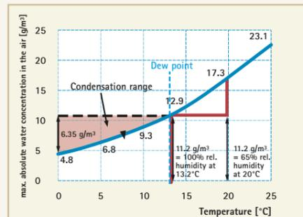
At an elevated relative humidity of 65% the dew point is already reached at 13.2°C. If the temperature drops to 0°C, significantly more condensation is deposited: 6.35 g/m<sup>3</sup>.
