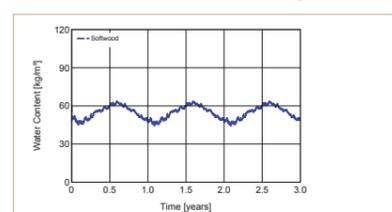
→ Insignificant increase in the moisture content of the 5 mm inner layer of wooden cladding
