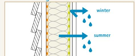
Humidity-variable airtightness membrane is diffusion-inhibiting in the winter, protecting the construction from condensation, but is able to become diffusion-open in the summer, allowing the construction to dry out
