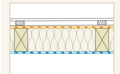
airtight on the inside and wind- and weathertight on the outside
