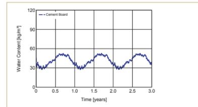
→ Insignificant increase in the moisture content of the cement-bonded boards
