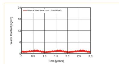
→ Insignificant increase in the moisture content of the 5 mm outer layer of thermal insulation
