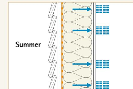
For constructions that are diffusion-inhibiting on the outside it is advisable to avoid diffusion-inhibiting material on the inside. Intelligent moisture management using INTELLO®, however, ensures a high potential freedom from structural damage.
