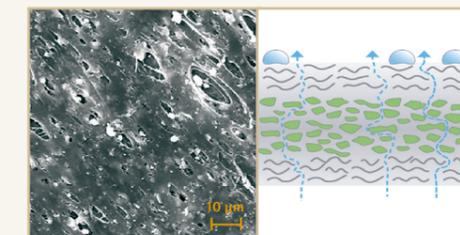
Microscopic detail of a porous membrane Passive diffusion transport
