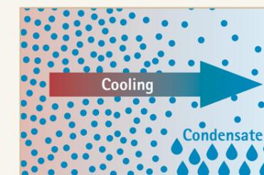
If warm air cools, condensate (condensation) may be deposited and there is a risk of structural damage and mould.
