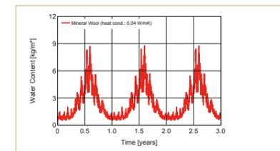
→ Moisture content of the 5 mm outer layer of thermal insulation rose to 9 kg/m<sup>3</sup>
