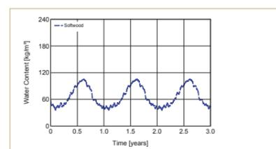
→ Moisture content of the 5 mm inner layer of wooden cladding rose to 110 kg/m<sup>3</sup>
