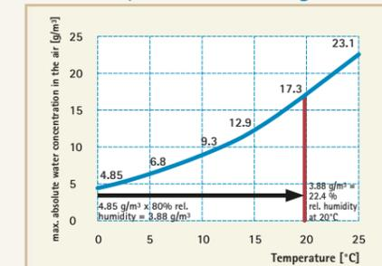
1 m<sup>3</sup> of air at 0°C and 80% relative humidity is heated to 20°C.
