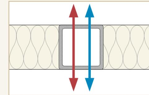
A steel support conducts the heat out of the building faster than the insulated compartment.
