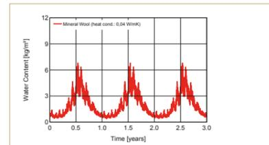
→ Moisture content of the 5 mm outer layer of thermal insulation rose to 6.5 kg/m<sup>3</sup>
