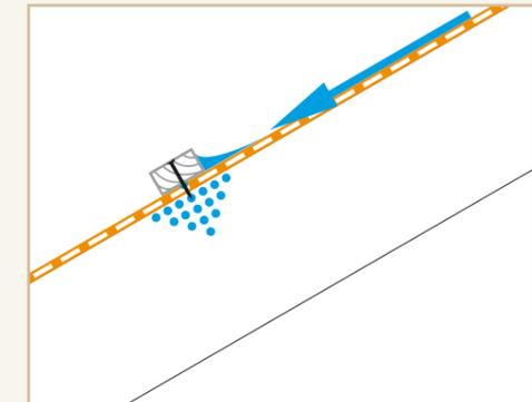
If roof battens are right on the roof underlay, the batten can act as a dam, resulting in ponding water that can then generate around the nails.
