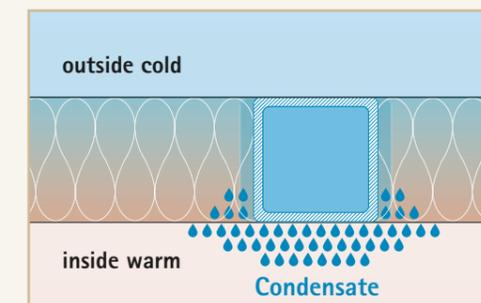
Thermal bridges contribute significantly to the growth of mould on the surfaces of building materials and to a reduction in energy efficiency.
