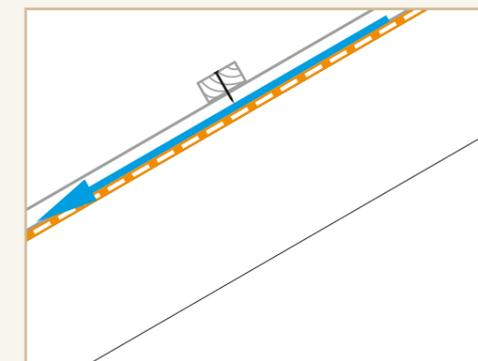
To ensure a watertight roof, at least counter battens should be used (battens along the rafters). Additional protection is provided by nail sealing tapes such as TESCON® NAIDECK under the counter battens.
