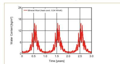
→ Moisture content of the 5 mm outer layer of thermal insulation rose to 15 kg/m<sup>3</sup>
