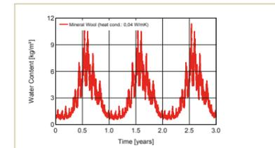
→ Moisture content of the 5 mm outer layer of thermal insulation rose to 11 kg/m<sup>3</sup>
