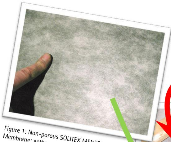
Figure 1: Non-porous SOLITEX MENTO® Membrane: active vapour diffusion -> dry enclosure, no condensation observed
