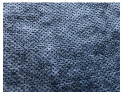
The **bottom microfiber fleece** protects the TEEE layer above from damage during construction.
